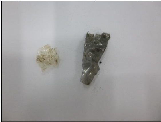
Figure 2 Enhancing the detection of transparent film plastic by graphite coating (right) alongside uncoated transparent film (left)
