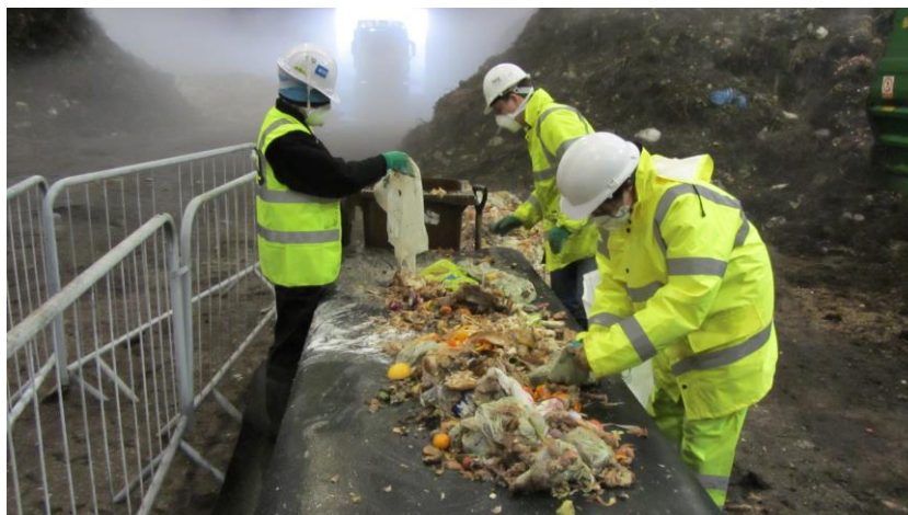
AfOR, TEG Environmental and Novamont staff sorting materials from a sample of bagged food wastes.
